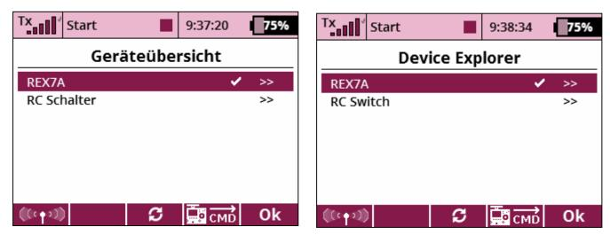
If you see REX6A, REX7A, REX10A or REX12A this will be an ASSIST receiver with integrated gyro stabilization system
